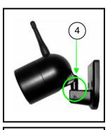
**5.** Point the camera in the desired position. Tighten the side screw to secure the camera to the Stand.
